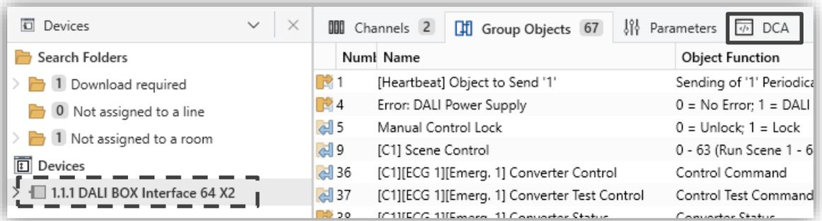
Figure 4. Project >> Device >> KNX-DALI Interface >> DCA Access
